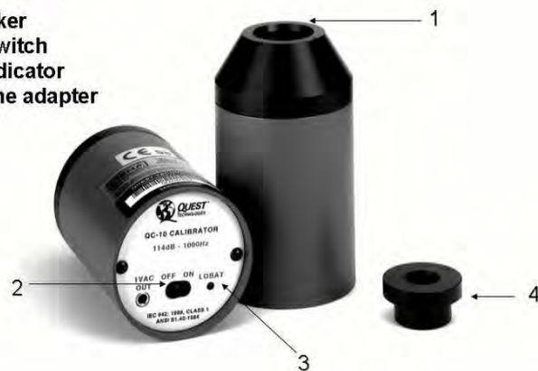
Figure 3.4 – Typical acoustical calibrator used for field calibration
