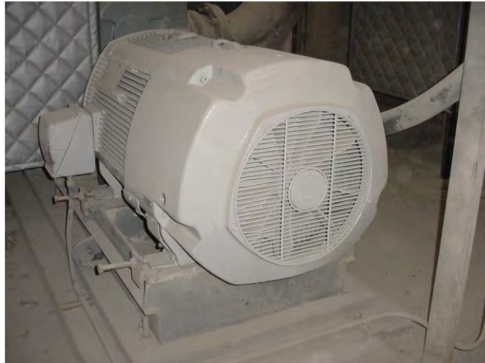
Figure 4.1 - Totally-enclosed fan cooled electric motor
