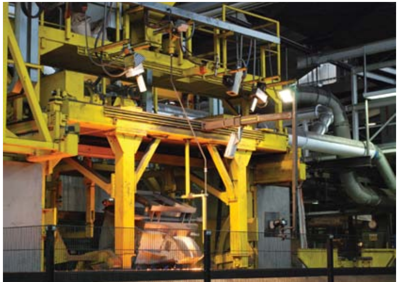
Federal-Mogul's Slow-Motion Casting Simulation technique using high-speed cameras to provide a more detailed analysis of mould filling, enabling precise optimization of the gating and feeder systems that control molten material flow
