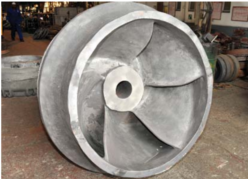
Last year Viking Foundry was tasked to cast an impeller for APE Pumps, part of a centrifugal water pump that is in operation at a local power station. The large and difficult impeller was cast in stainless steel CA15. Gross weight of the casting was 3 250 kilograms with a final nett weight of 2 180 kilograms. The casting had a diameter of 1650 mm and a height of 1200 mm with a vane thickness of 50 mm, a heavy centre boss and outer wall thickness of 110 mm
