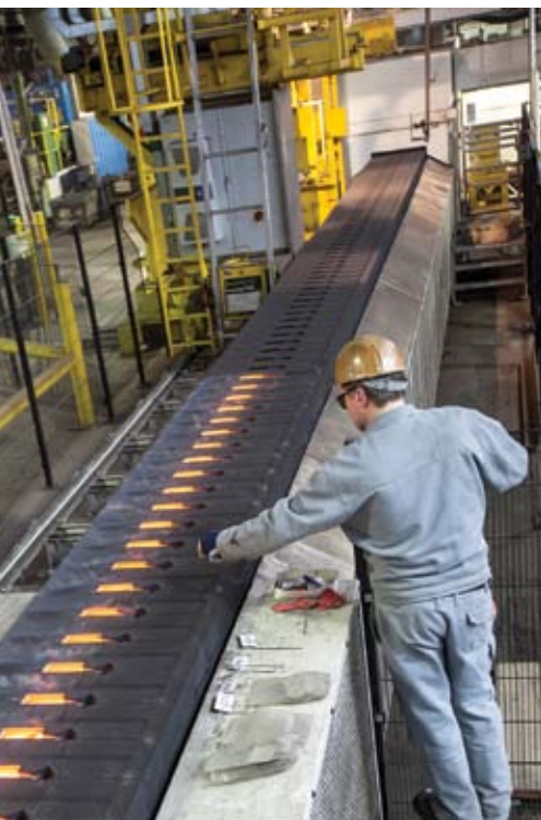
Casting a new steel alloy for piston rings at Federal-Mogul's Burscheid, Germany, ferrous foundry
