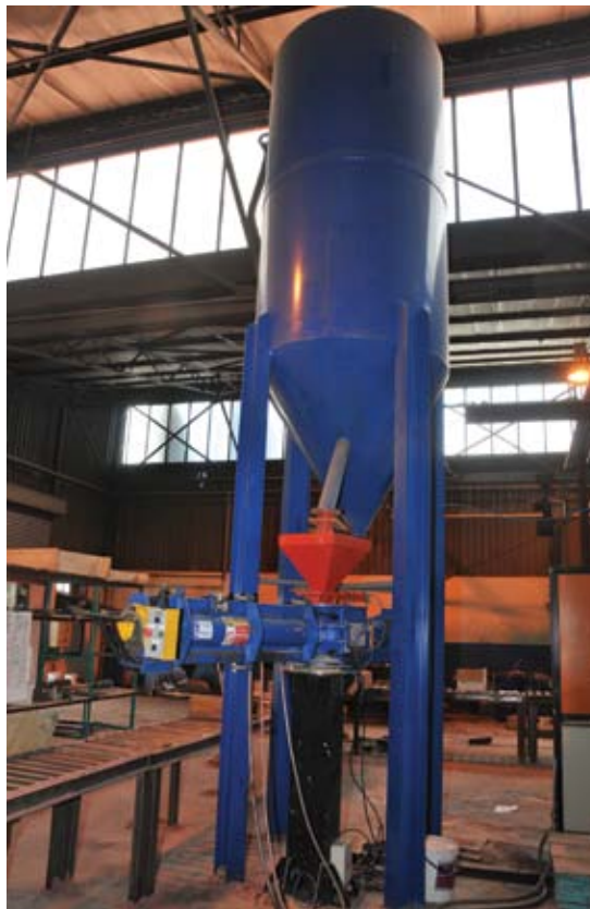
Lauds Machinery supplied a Lauds 3000 temperature sensitive no-bake blending unit. The unit supports the Lauds LT6-12TPH pivotal continuous mixer. The system is fed with a 10mt bulk fed hopper
