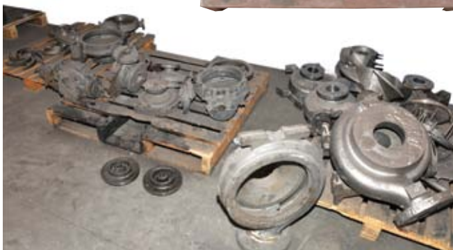
Various castings manufactured by Rapid Allweiler for the company's own use
