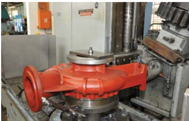
A pump being machined
