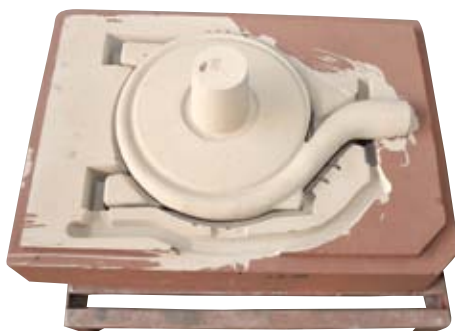
Resin sand mould before closing and casting
