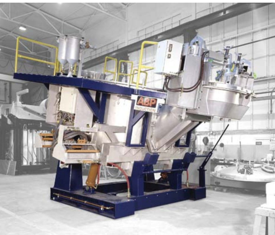
The ABP pouring furnace PRESSPOUR® type OCC pouring with two stoppers
