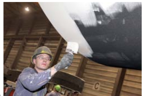
The correct mixture of furan resin is an indispensable success factor for large-scale casting
