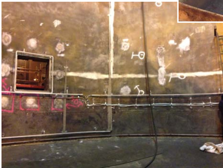
Arrangement of the Savedry sensors in a prefabricated rack at the tap hole and circumference of a DC arc furnace
