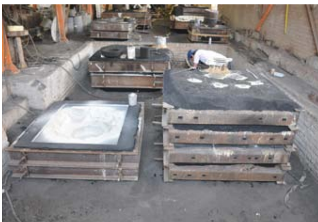
A pit where larger castings are poured
