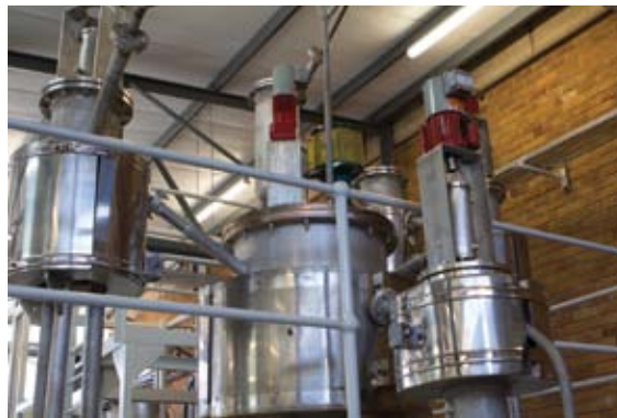
A view of the main reduction unit of the titanium pilot plant
