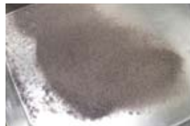
Silica sand and chromite (prior to separation)
