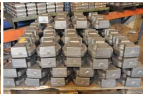
Castings ready to be transferred to the machine shop
