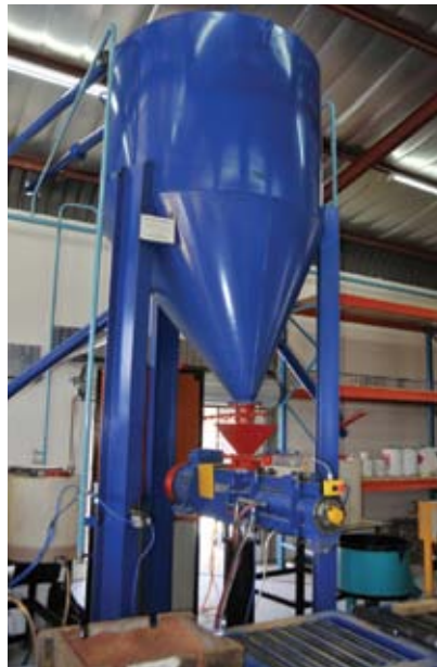
The Lauds I-3TPH high speed continuous mixer with a Lauds Auto-Blend 3000, which is a temperature sensitive blending dosing system for the mixer
