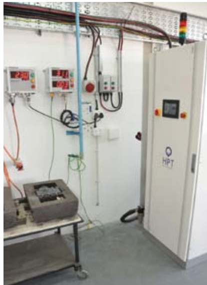
The HPT furnace is equipped with the latest IGBT based induction power supply unit, which offers lower energy consumption. It is located next to the latest measuring and testing equipment available
