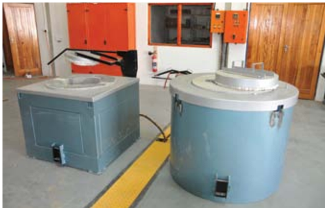
The two 50 kilogram furnaces installed for non-ferrous melting
