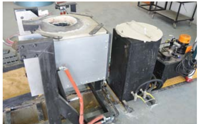
The 50 Kg cast iron induction tilt melter custom designed and manufactured in South Africa by HPT
