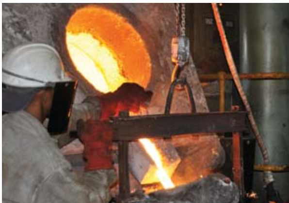
Metal being transferred to a ladle. The foundry makes use of two one-ton Inductotherm melting furnaces with VIP controls
