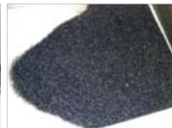
Reclaimed chromite sand (after separation)
