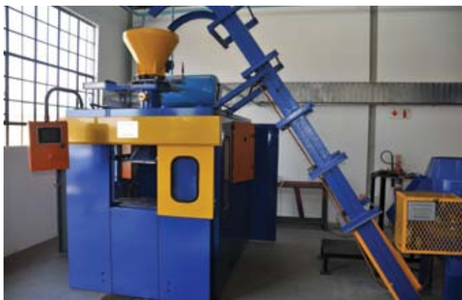
The Lauds 6L hydraulic jobbing cold box core blower complete with the Lauds vertimix batch mixer and pump set which feeds directly into the Lauds skip hoist delivering mixed resin cold box sand to the core blower on a fully automatic basis
