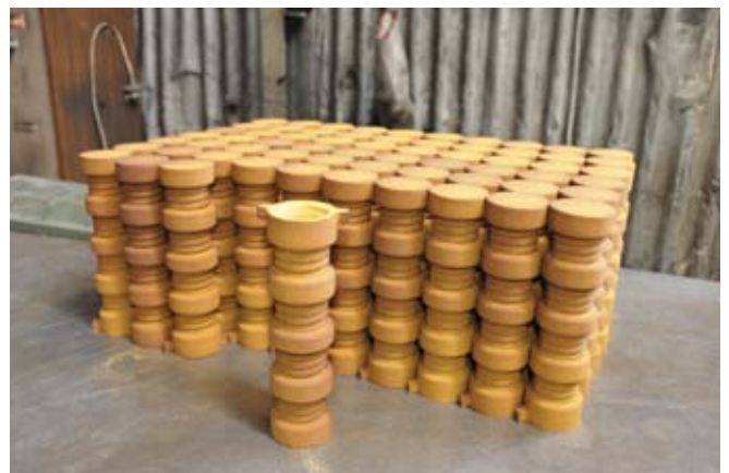
Shell cores for the internal thread of a product. After casting the thread never requires any further work
