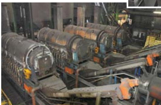
The four new LNG (liquid natural gas) gas fired quench furnaces, each with an increased capacity of 20%
