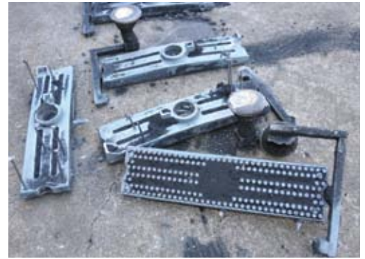
Right: A burner body that required many trials before the company succeeded in manufacturing a casting to the client's satisfaction. One of the difficulties was due to the escape of gas from the core. The company's motto is that they rather try to fail than fail to try
