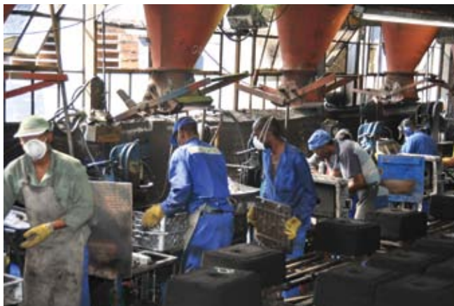
Zimmerman jolt squeeze moulding machines
