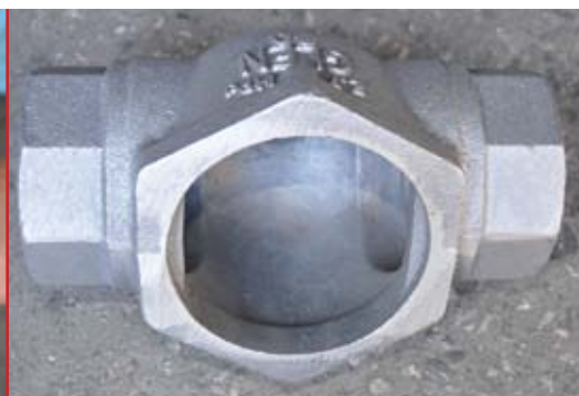
A valve body casting with internal section done with shell core
