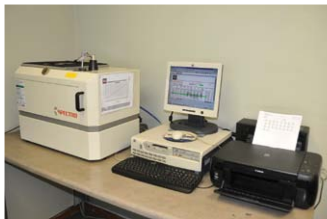
The quality of the metal is of top priority at Malleable Castings and here they utilise a Spectro spectrometer, which is housed in a climate controlled laboratory
