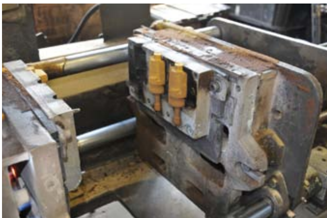
All shell cores are produced in house on 14 shell core machines
