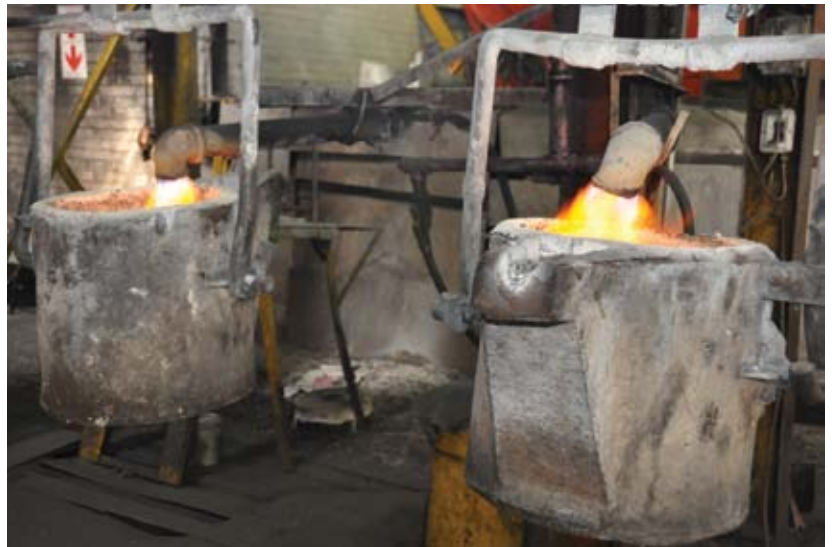
150 Kg ladles being preheated for the next tap
