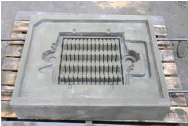
Furane sand mould before coating and closing
