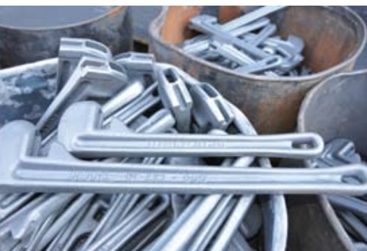
Casting sizes and weights range from 0.1 kilogram to 30 kilograms, shell cores are produced in-house to satisfy the full range of castings produced and the pattern plate dimensions are 460mm x 160mm and 500mm x 160mm
