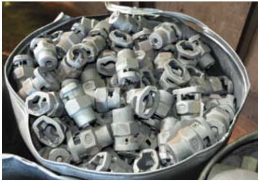
Left: Spud type castings post knock off and ready for fettling
