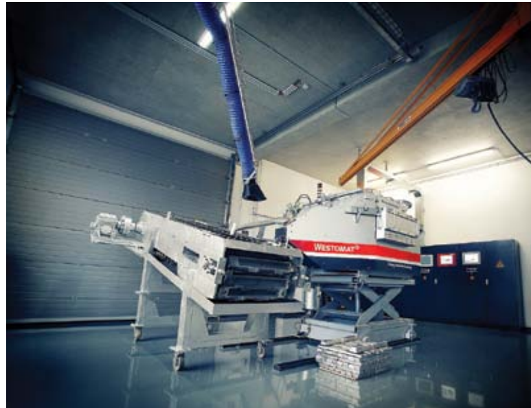
Fully functional: the Westomat dosing furnace at the Wiehl Pilot Plant Centre allows extensive practical customer training courses to be held under real-life foundry conditions
