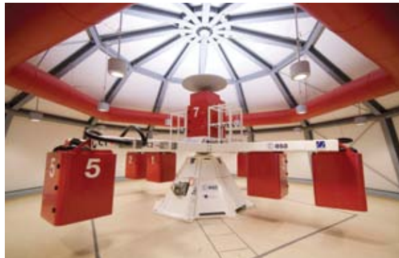
The Large-Diameter Centrifuge at the European Space Research and Technology Centre at Noordwijk, The Netherlands. The rotation of the LDC creates a hypergravity field inside each gondola. The LDC has an 8-m diameter, with four arms that support up to eight gondolas (two per arm), with a maximum payload of 80 kg per gondola. In practice, six gondolas are available, plus one gondola in the center for control or reference experiments
