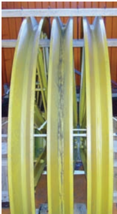
KEW Foundries supplied a copper and gold mine in Mongolia with three 10-foot sheave wheels that will operate in extreme climatic conditions
