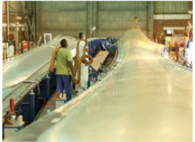
The sleek surface of Africa's first locally produced blade for a 2.5MW wind turbine is revealed as one views it from above. The blade is 50 metres long and is relatively light for its size at a weight of 12 tons, because it is made from lightweight materials, including balsa wood and fibreglass. At 50 metres from the tapered tip to the round, hollow end, I-WEC's first multi-megawatt wind turbine blade is longer than an Airbus wing. Each wind turbine will be fitted with three of these blades. The turbine will measure 130 metres high from bottom to top, with the length of the blade included
